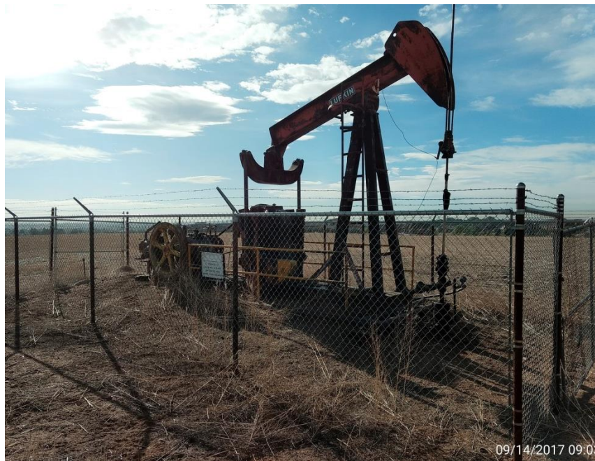
Wellhead, pumping unit, and prime mover
