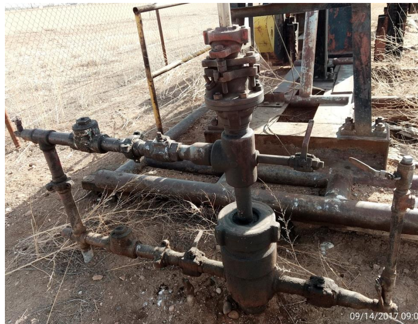
Wellhead detail, Tubing open, casing closed, casing backside tied into 1" buried line.
