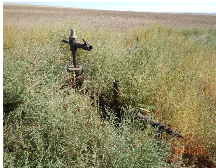
Photo #16 – Uncapped and unplugged valves plumbed to wellhead.
