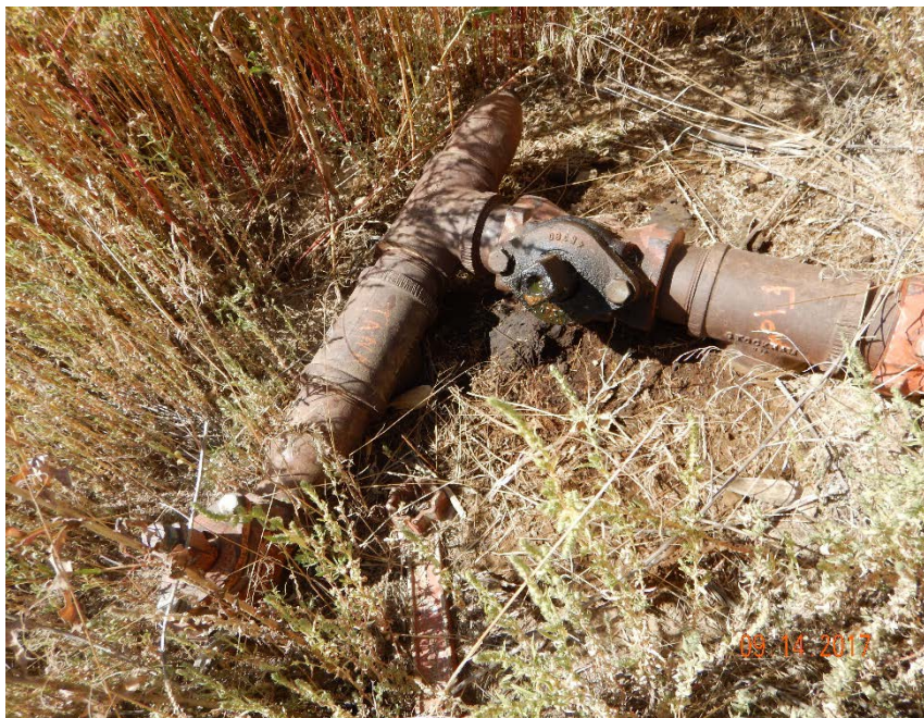
Photo #7 – Exposed flowline manifold north of buried concrete vault has localized accumulations of oily waste.
