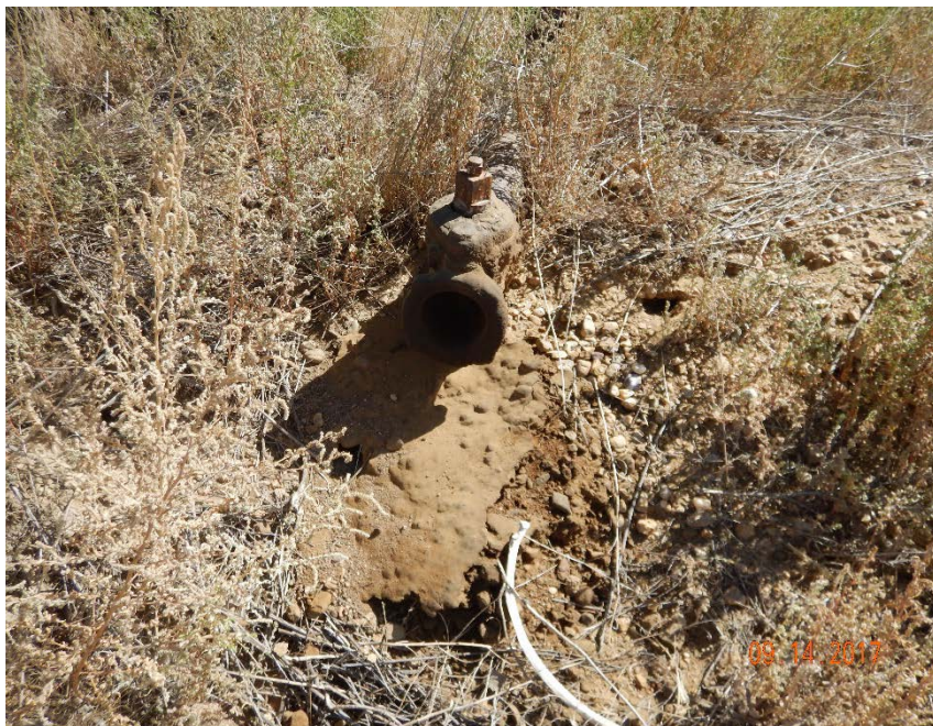
Photo #1 – Historical accumulation of oily waste at crude oil tank loadout. Note: loadout lacks secondary containment device.
