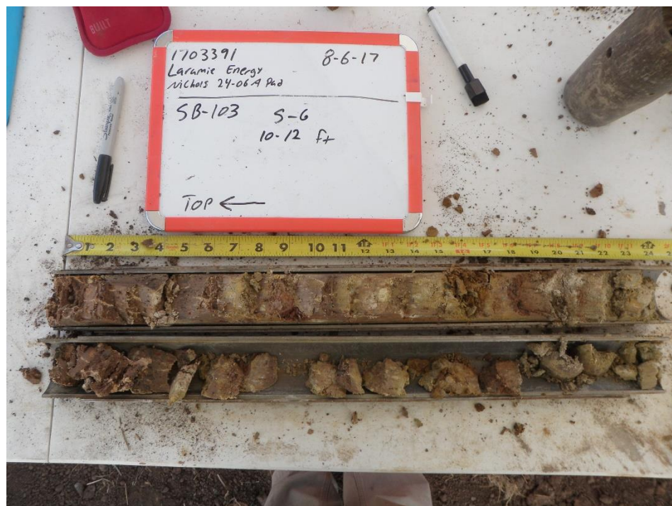
Photo No. 14 – Boring SB-103 10-12 feet, clay.
