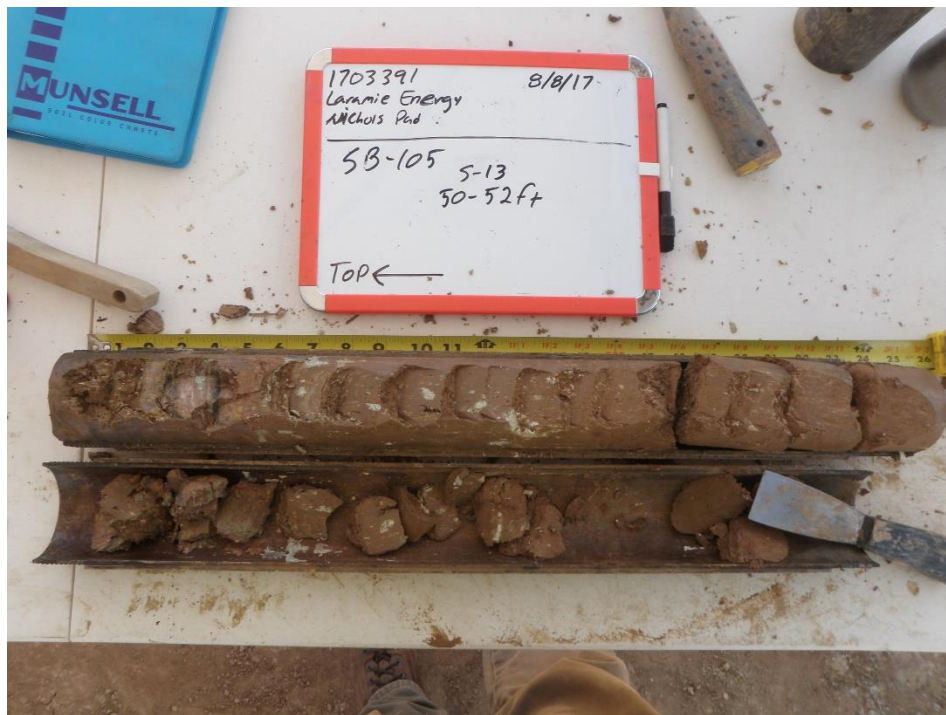
Photo No. 16 – Boring SB-105 50-52 feet, clay.
