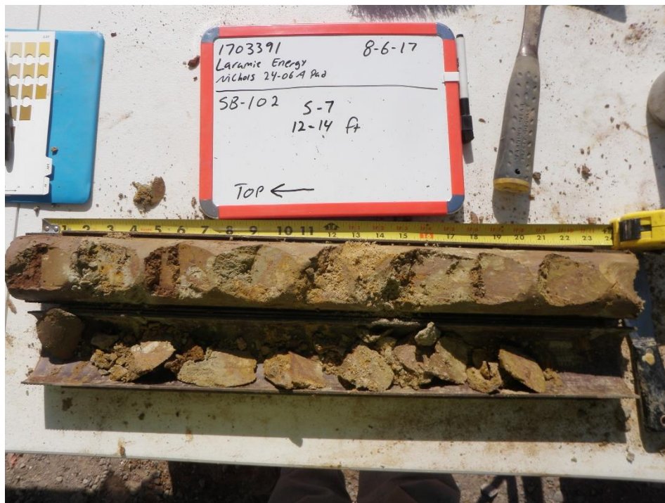
Photo No. 12 – Boring SB-102 14-16 feet, clay.
