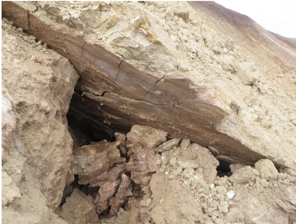
Photo No. 3 – Close-up of planar slope failure surface.
