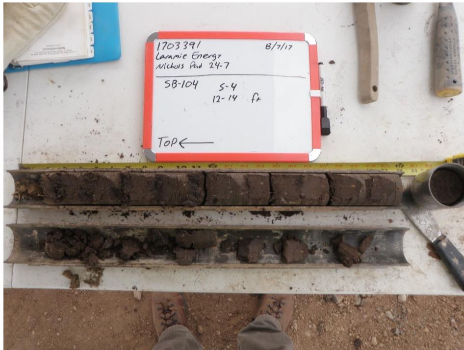
Photo No. 15 – Boring SB-104 12-14 feet, clay.
