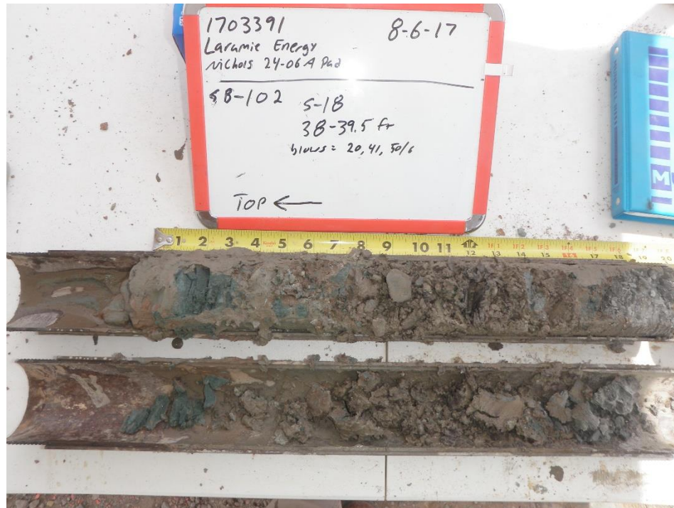
Photo No. 13 – Boring SB-102 38-39.5 feet, likely top of weathered bedrock. (Relict bedrock structure noted)
