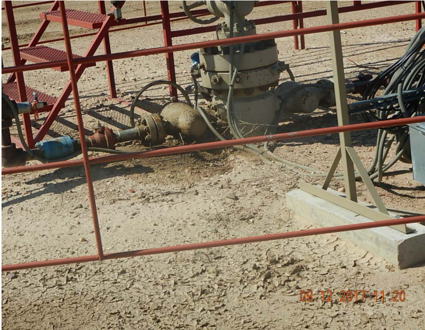
Photo 3: Stained soil at wellhead
