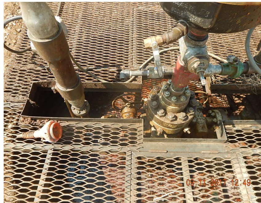
Photo 7: Stained soil, oil in cellar.
