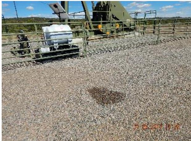
**Photo 5: Impacted soil and gravel. Previous inspection.**
