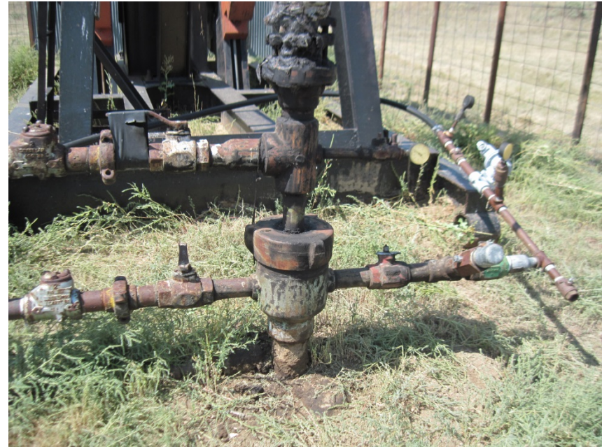
WELLHEAD STAINED SOIL
