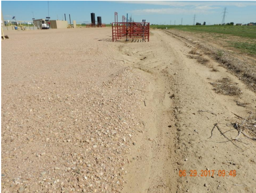
Photo 1. Photo taken June 29, 2017 from the northeast location, facing North. Appears stormwater and/or irrigation water run-on is flowing onto location which then travels across the eastern location through the wells. Gully erosion is occurring along the eastern location and off location.
