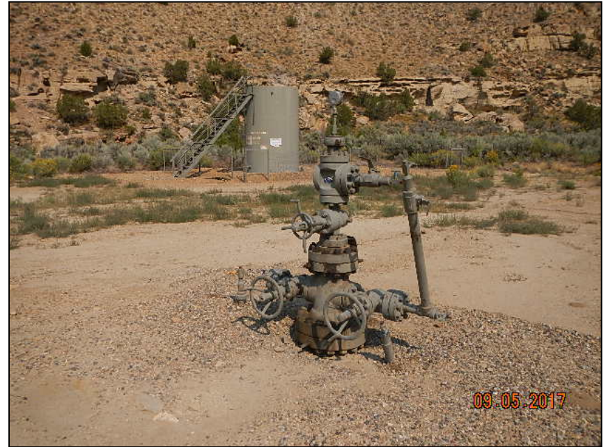
Photo 2. Wellhead not connected.
