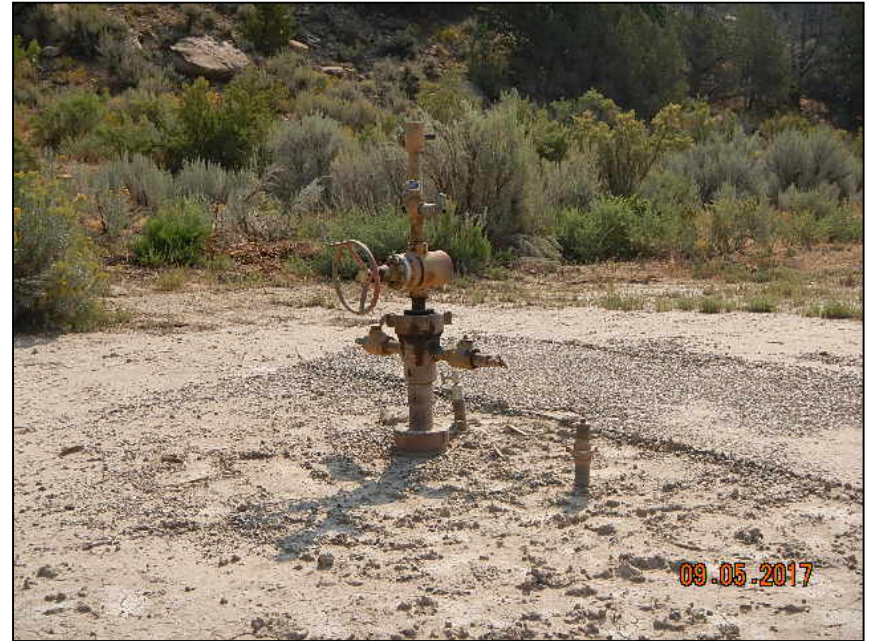
Photo 2. Wellhead not connected.
