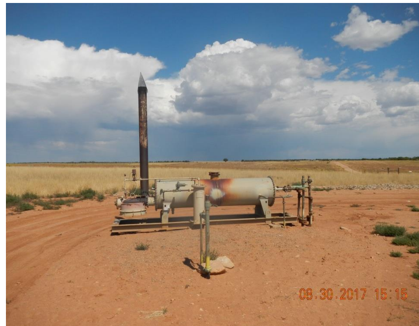
Horizontal heater treater.
