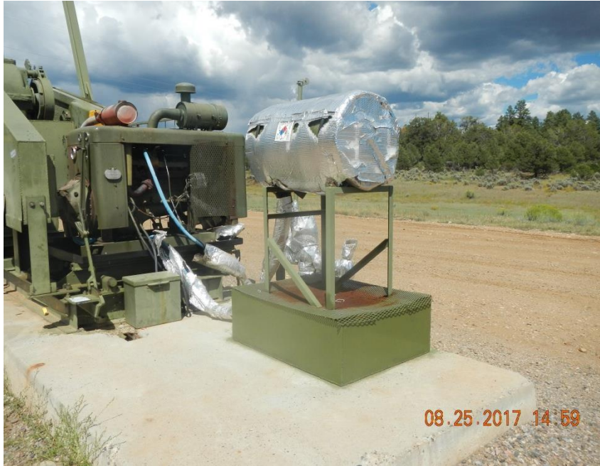
Lube oil container with secondary containment.
