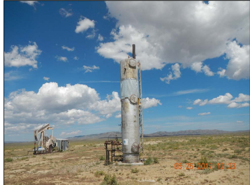
Photo 4. No wildlife protection on separator exhaust.
