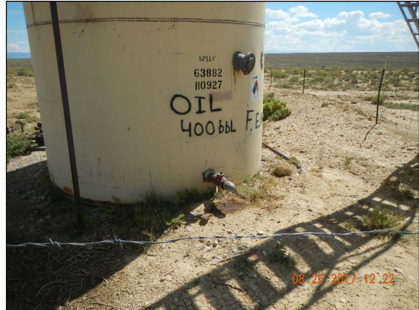
Photo 2. Stained soil at tank loadout.
