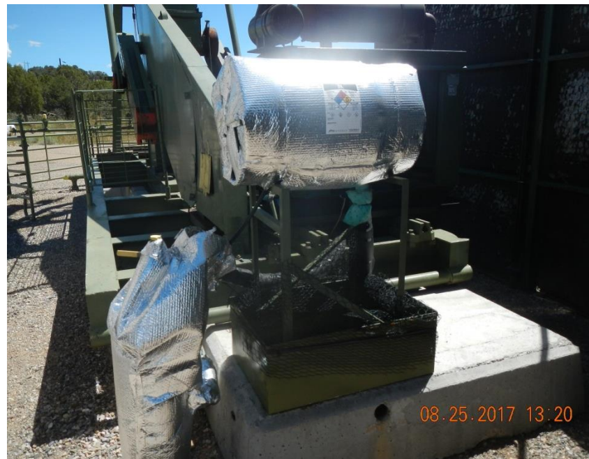
Secondary containment for lube oil container.
