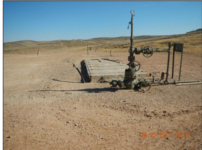
Photo 2. Unused riser at wellhead. Pump jack base.
