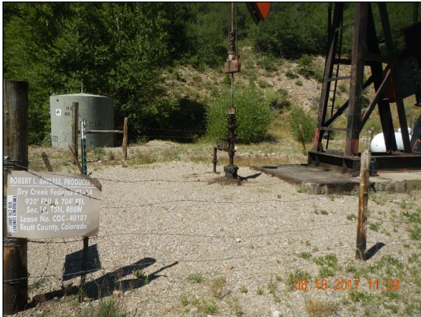
Photo 1. Stained soil at wellhead.
