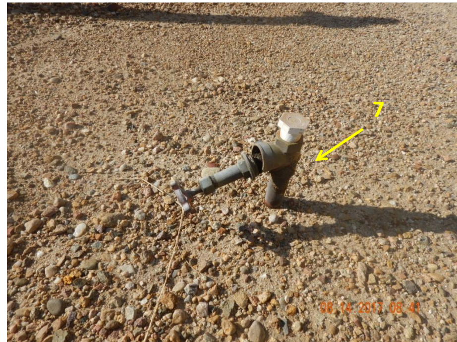
Photo 6: Photo taken from the central area of the battery facility. Photo shows risers at the battery. Inspection doc. #682502037 required operator to comply with reclamation requirements and the 2017 Flowline NTO to remove the risers. Riser seen here does not appear to be in proper function condition and needs to be removed.
