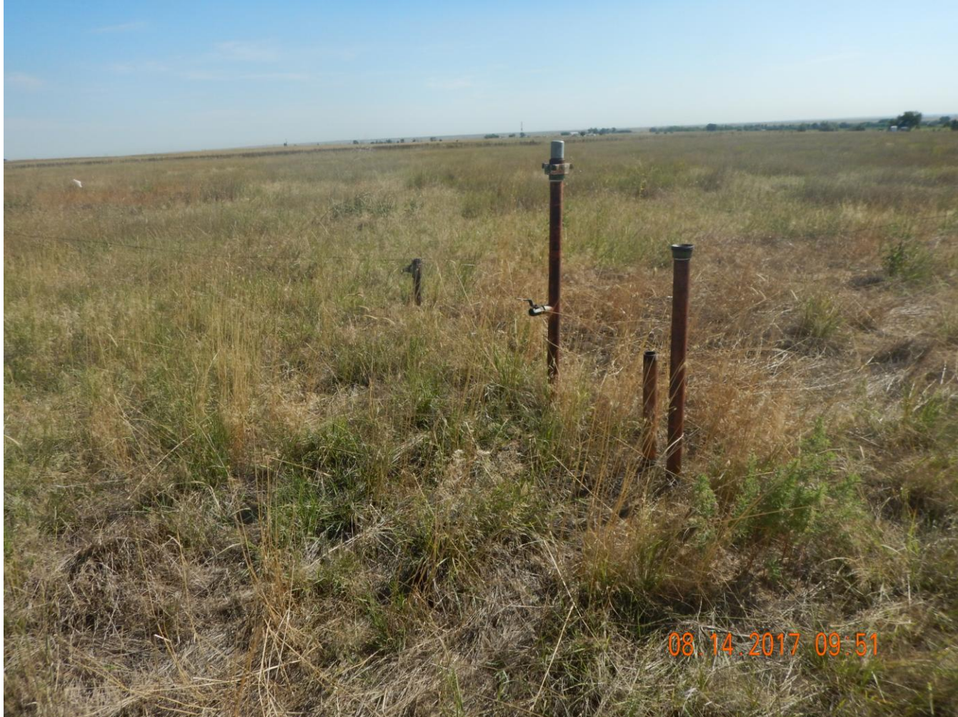
Photo 1: Photo taken from the former tank battery location, facing northeast. Previous inspection doc. #682502071 required operator to remove risers in accordance to the 2017 Flowline NTO. Risers still remain at the battery location and are now subject to reclamation requirement for removal.
