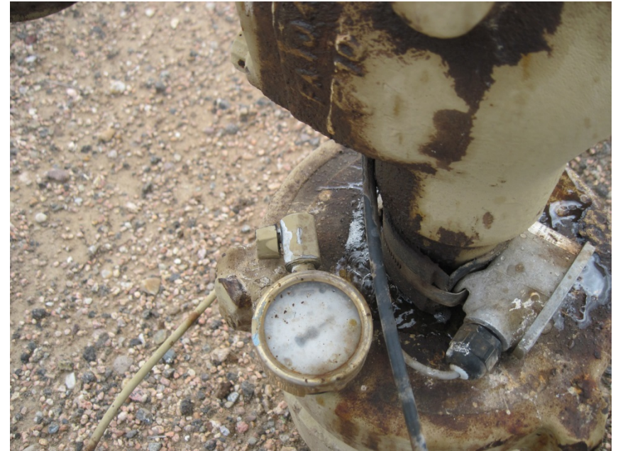
WELLHEAD LEAKING AT CAP
