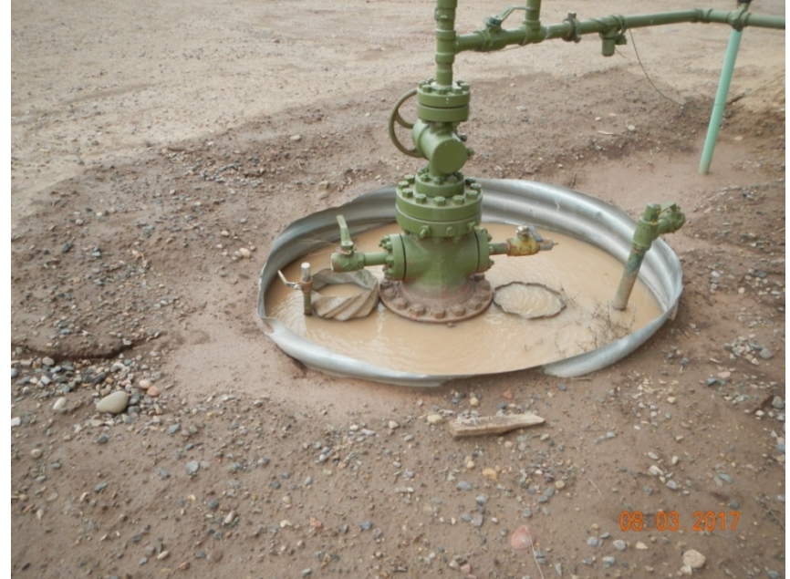
Photo 4: View of open cellar at wellhead.
