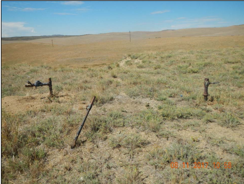
Photo 2. 2 -2" steel risers and 1 – 1" steel riser.
