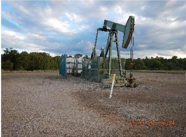
**Photo 17: Photo of pump jack with sound walls taken from SE corner of location.**
