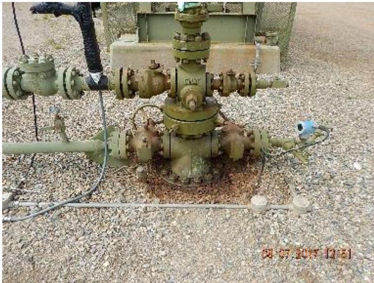
Photo 11: Impacted soil at wellhead.
