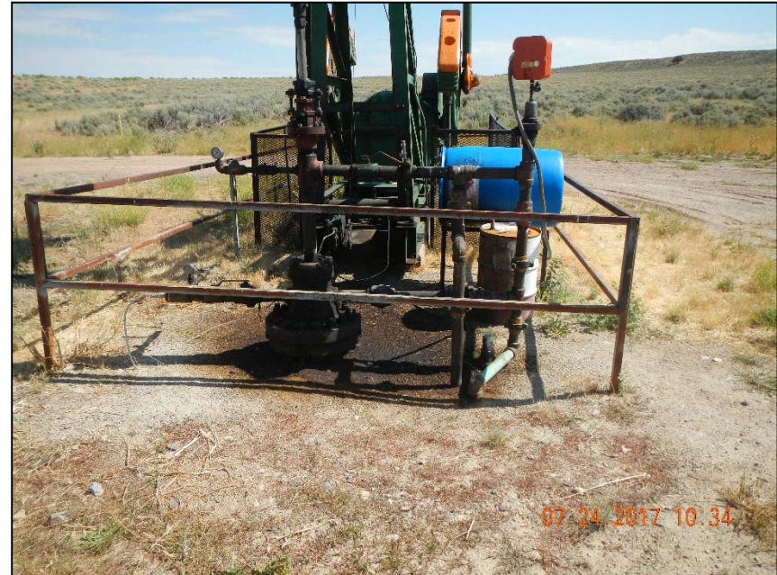
Photo 3. Stained soil at wellhead. Containers without secondary containment on right side of picture. 1 – 2" steel riser.
