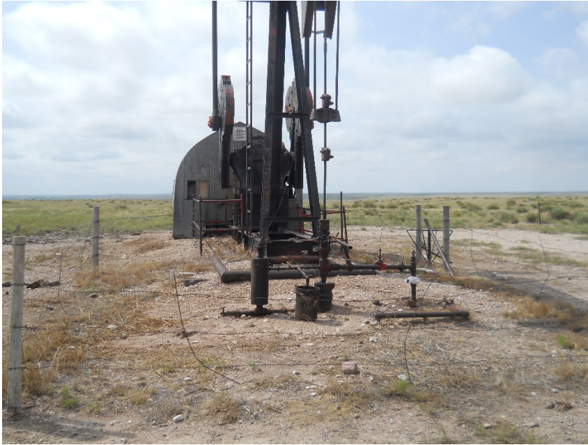
Pump jack looking south, open top container containing fluid with no wildlife protection
