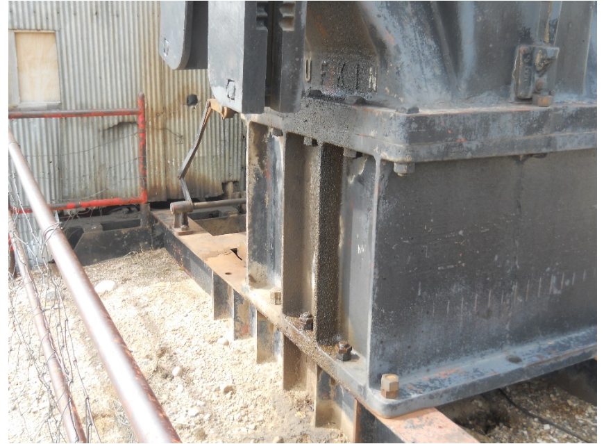
Leaking gear box on east side of pump jack
