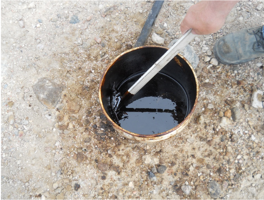
Open top container for pump jack blowdown, contains lube oil, has a dead bird in it, no wildlife protection
