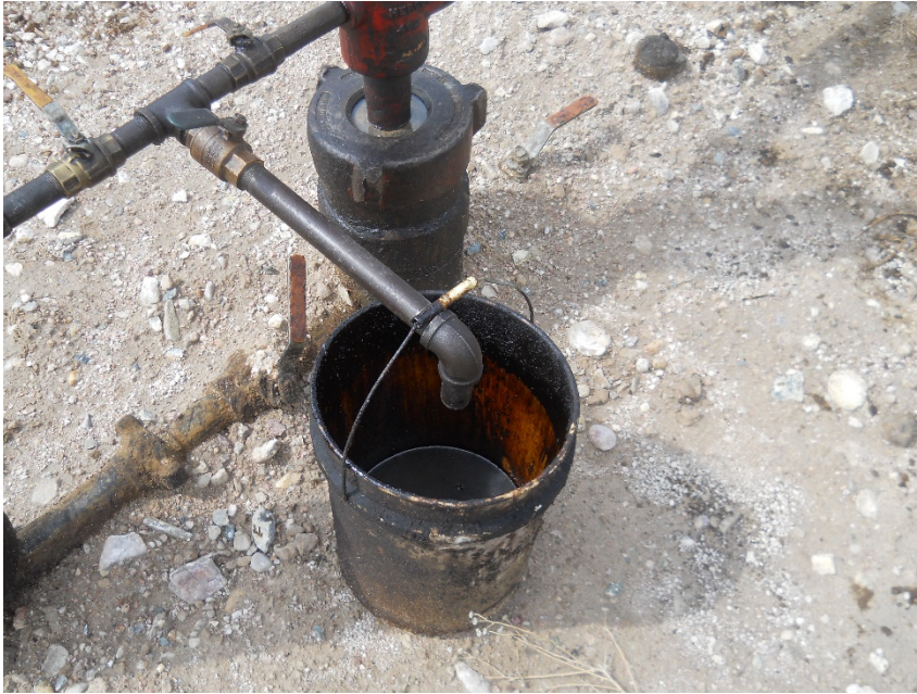
Open top container north side of wellhead containing fluid with no wildlife protection
