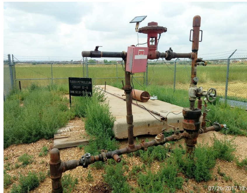
Wellhead, Corrective action: Emergency contact info not updated, scrubber not removed.
