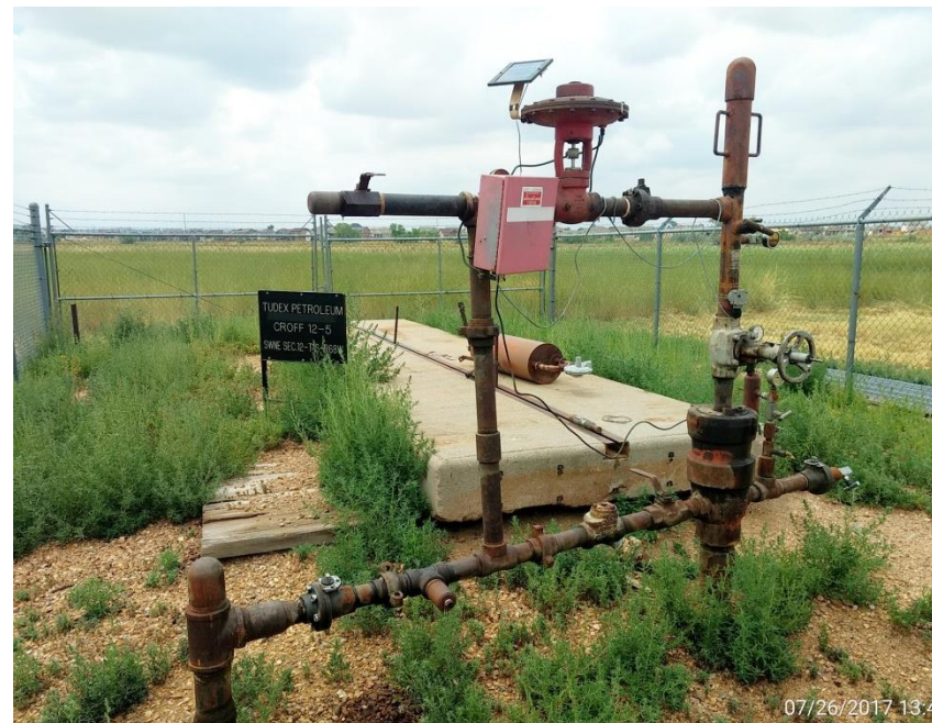
Wellhead, Corrective action: stained soil not remediated.
