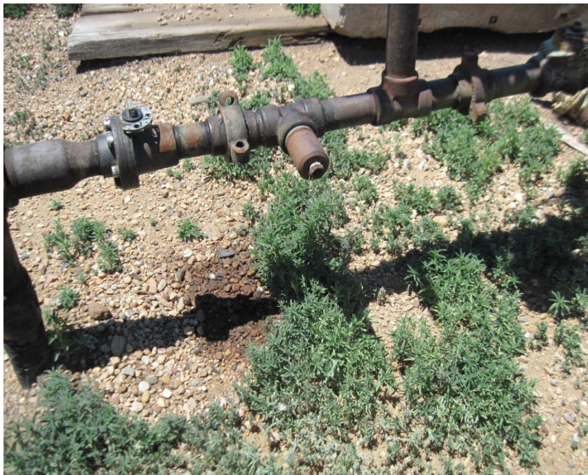
Stained soil at wellhead from 6/20/2017 inspection
