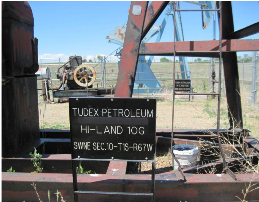
Wellhead signage, from 6/20/2017 inspection photos. Corrective action: No emergency contact info.
