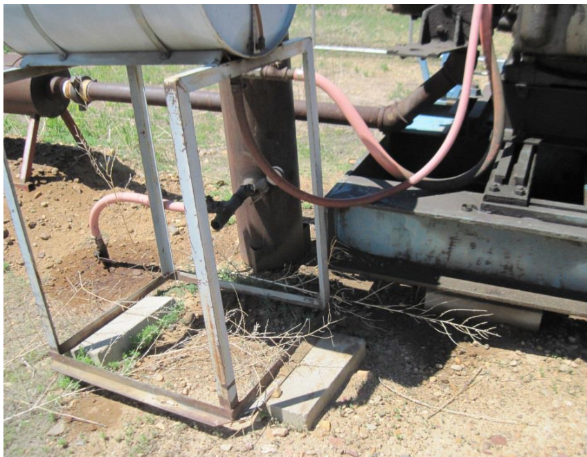
Pumping unit long run drum, 6/20/2017 inspection photo, Corrective action, stained soil.
