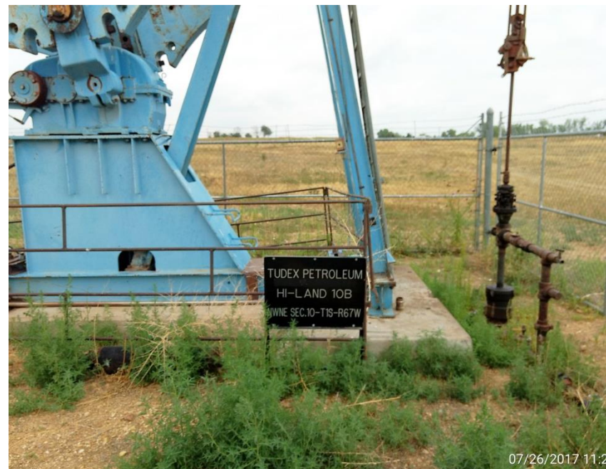
Wellhead signage, Corrective action: emergency contact info not updated.
