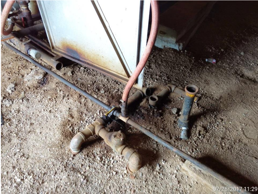
Inside of separator housing, Corrective Action: stained soil, Note: Unidentified risers.
