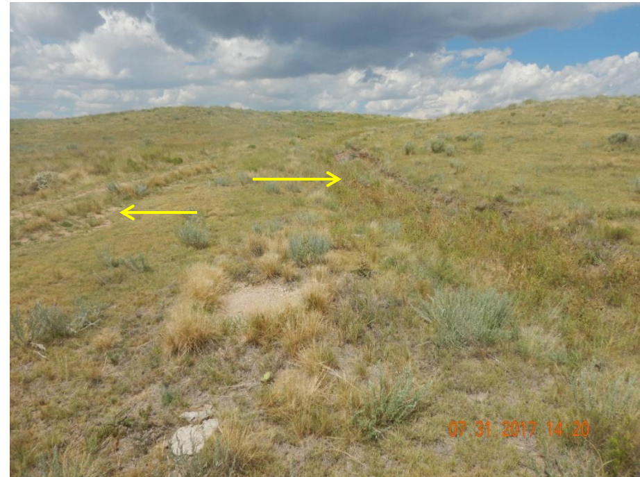
Photo 6: Photo taken from the access road on the north end of the location, facing north. Photo access road has not been re-contoured or re-graded. Arrow to the left shows road, arrow on right shows a ditch parallel to where the road travels uphill.
