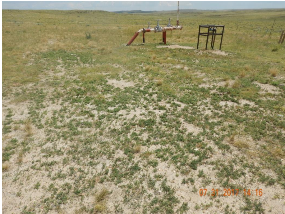
Photo 1: Photo taken from the location, facing south. Photo shows large areas of the location where vegetation is not progressing towards reclamation requirements. Vegetation seen is predominantly undesirable weedy plant species such as Kochia and Russian thistle. Photo also shows pipe equipment remaining on location.
