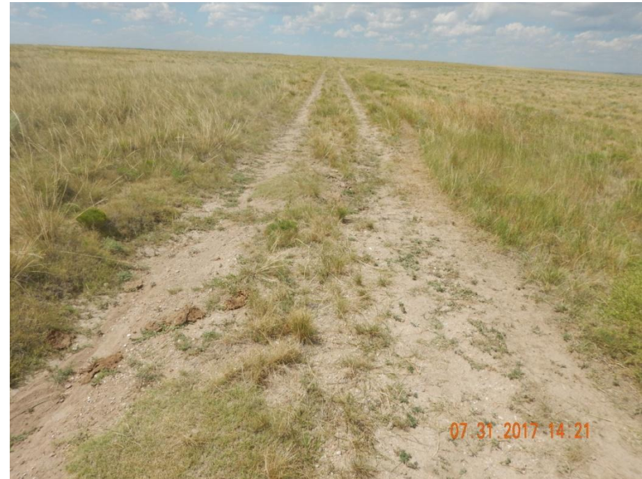
Photo 8: Photo taken from the access road on the north end of the location, facing north. Photo shows access road has not been re-contoured or re-graded.
