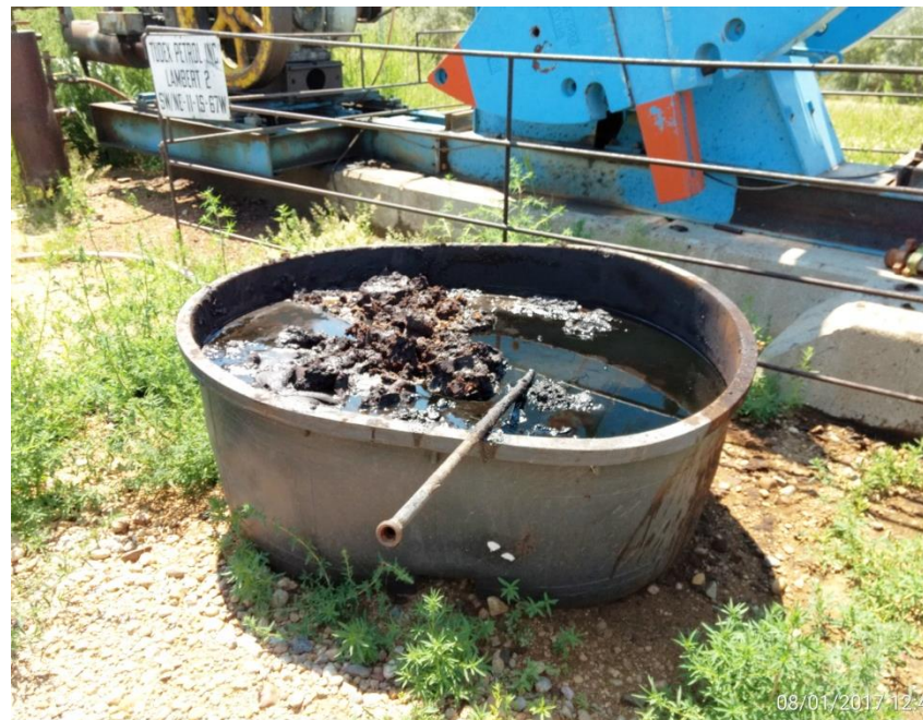
Pumping unit, Corrective action: Container full of paraffin and fittings not remediated.
