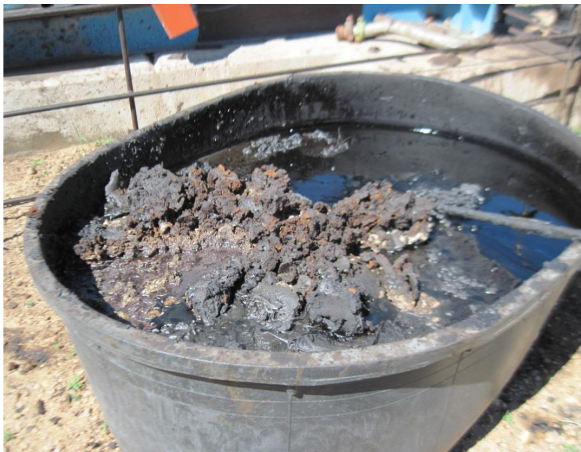
Pumping unit from 6/20/2017 inspection, Corrective action: fittings and container full of paraffin.
