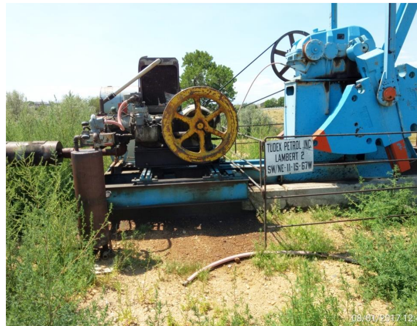
Pumping unit, Corrective action: Stained soil around prime mover and pumping unit frame not remediated.
