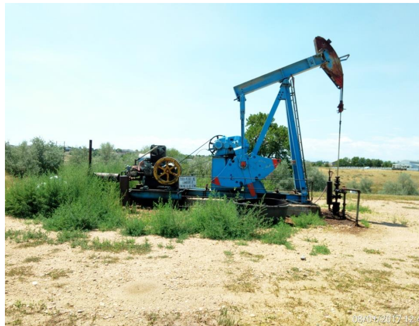
Wellhead, pumping unit, and prime mover.
