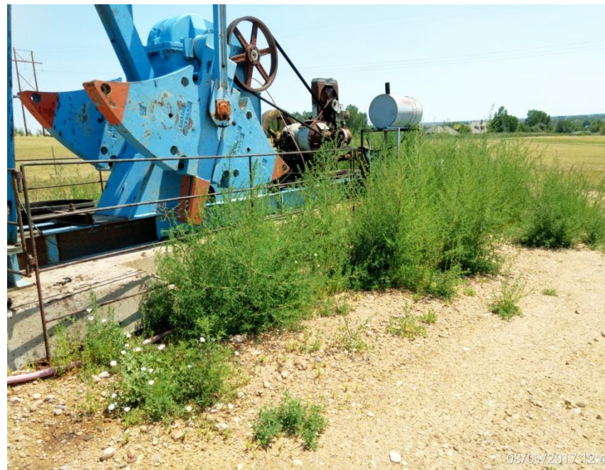
Wellhead, pumping unit, and prime mover, Corrective action, no signage, overgrown weeds.
