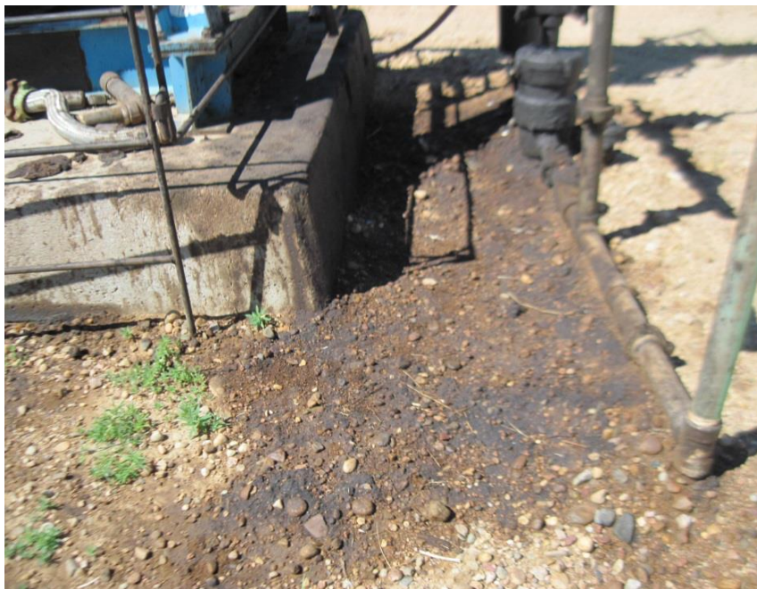
Wellhead from 6/20/2017 inspection, Corrective action: Stained soil.
