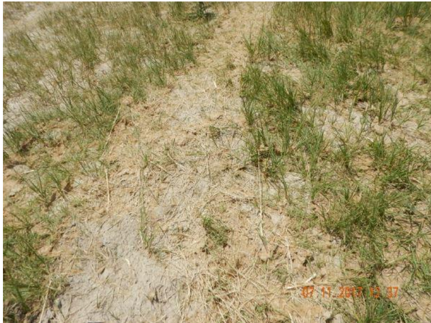
Photo 10. Close up photo taken just beyond the corner of the fence, illustrating stormwater runoff appears to be washing hydromulch material and sediment off location.
