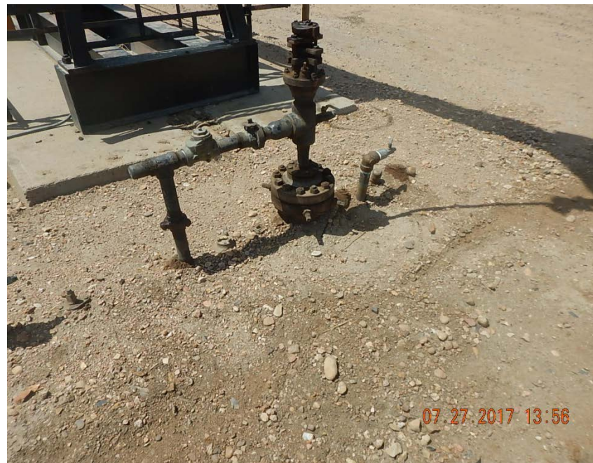
Photo 1: Stained soil at wellhead
