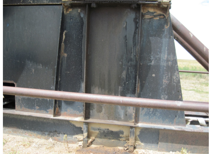
Stained soil from leaking gear box
