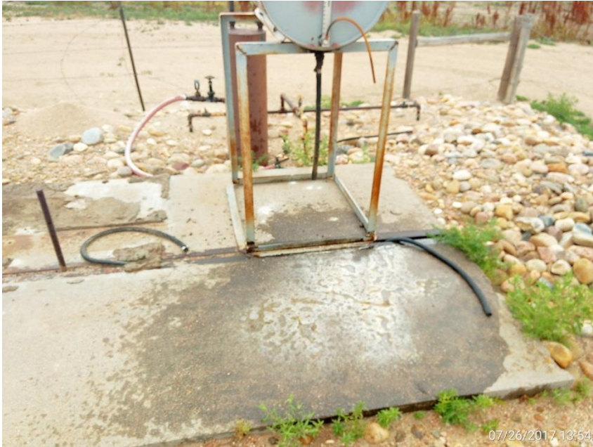
Long run oil drum Note: fluid spilled on concrete pumping unit base.
