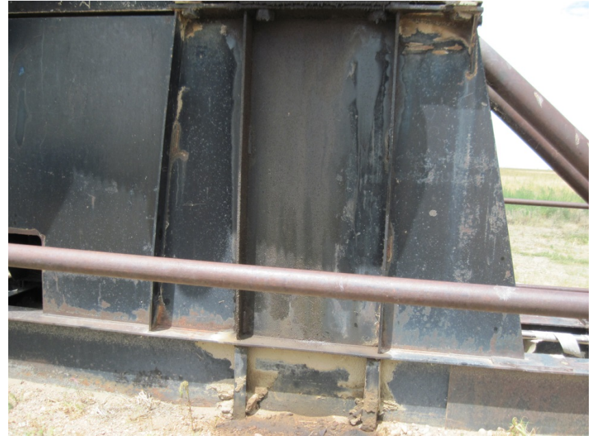
Stained soil from leaking gear box
