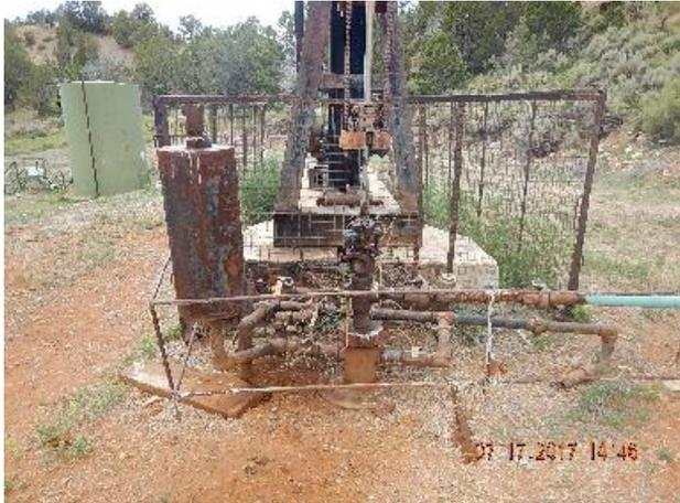
**Photo 5: Impacted soil at wellhead and loose pipe and fittings.**
