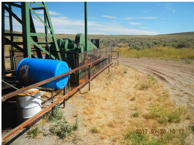
Chemical containers not in secondary containment.
