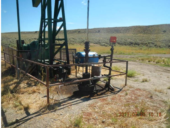
Stained soil around well head.
