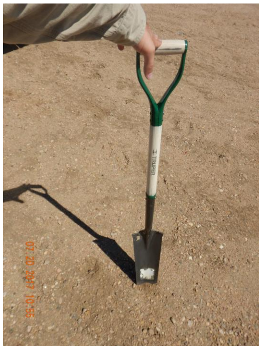
Photo 5: Photo taken from the tank battery location. Inspector made attempts to conduct a soil pit to test for compaction concerns. Inspector was unable to dig more than a couple inches. Location has not had compaction alleviation.
