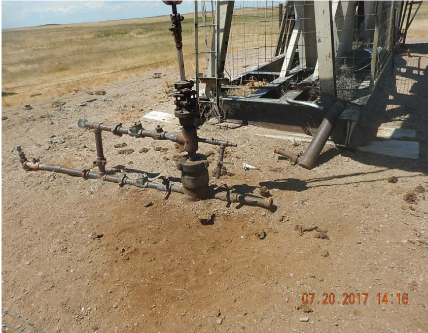
Photo 1: Bradenhead not plumbed to surface
