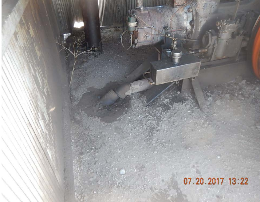
Photo 3: Stained soil at exhaust
