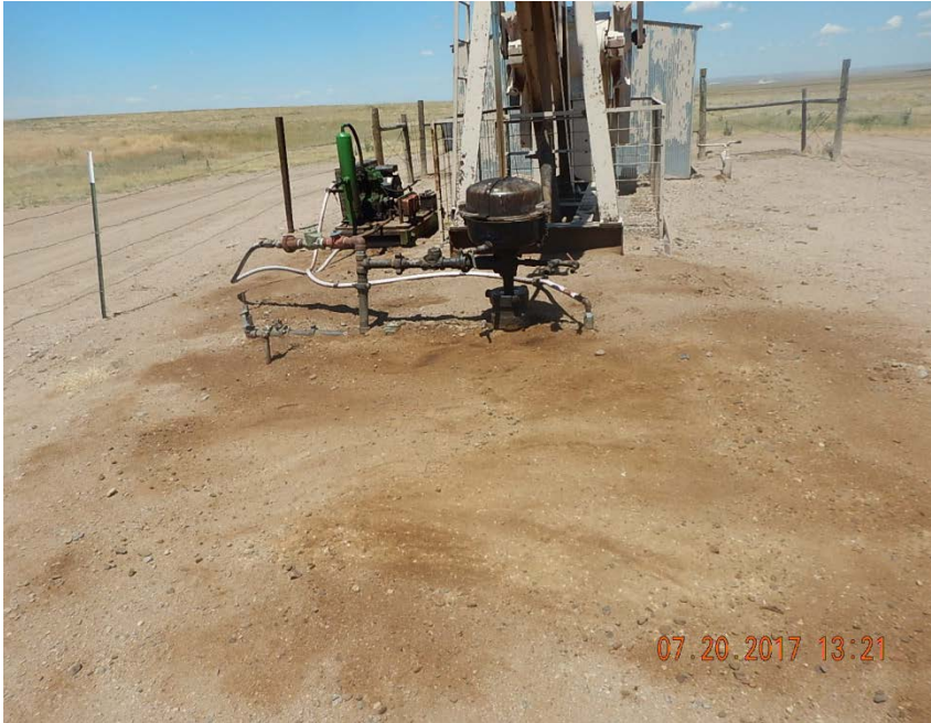
Photo 1: Stained soil at wellhead
