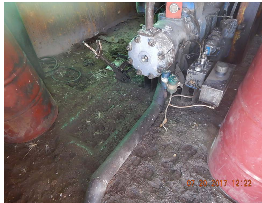
Photo 10: Stained soil in engine house.
