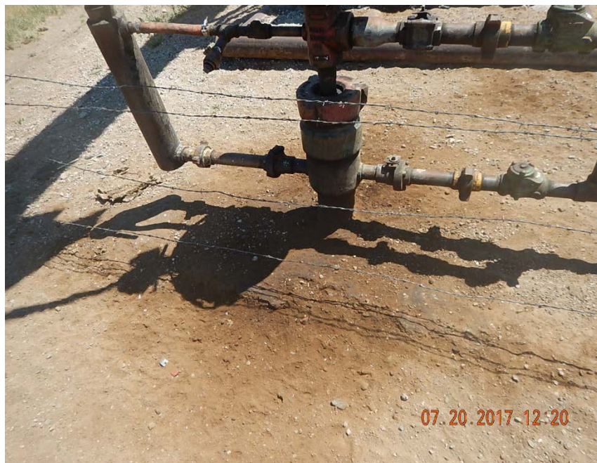
Photo 9: Stained soil at wellhead. No bradenhead at surface.
