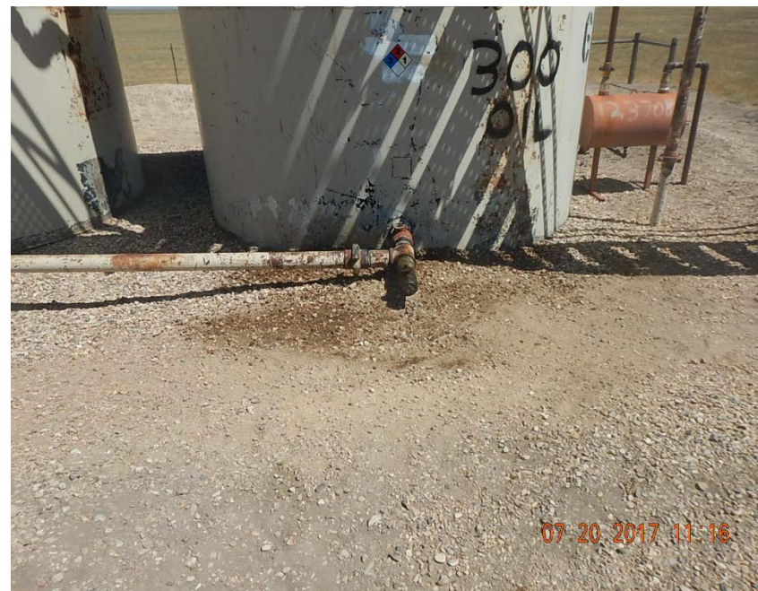
Photo 2: Stained soil at loadout
