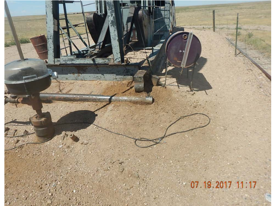
Photo 4: Stained soil at pump jack
