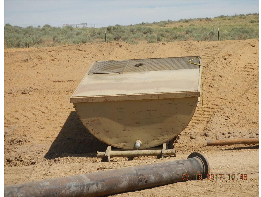
Photo 8 Cement cleanout apparatus.
