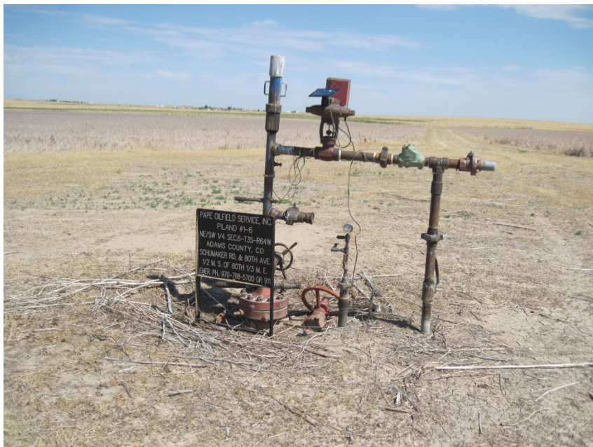
wellhead, intermitter controller
