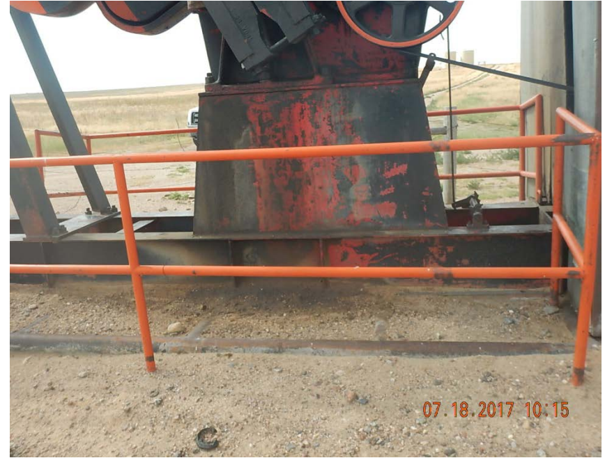
Photo 2: Stained soil at pump jack
