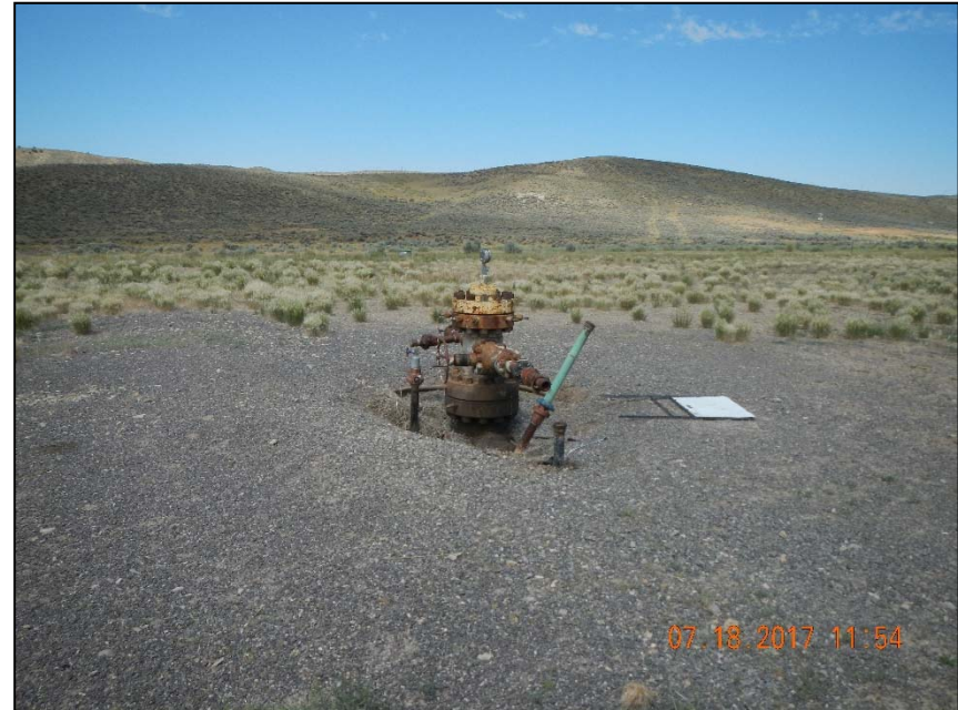
Photo 3. Unused 2" steel risers at wellhead.
