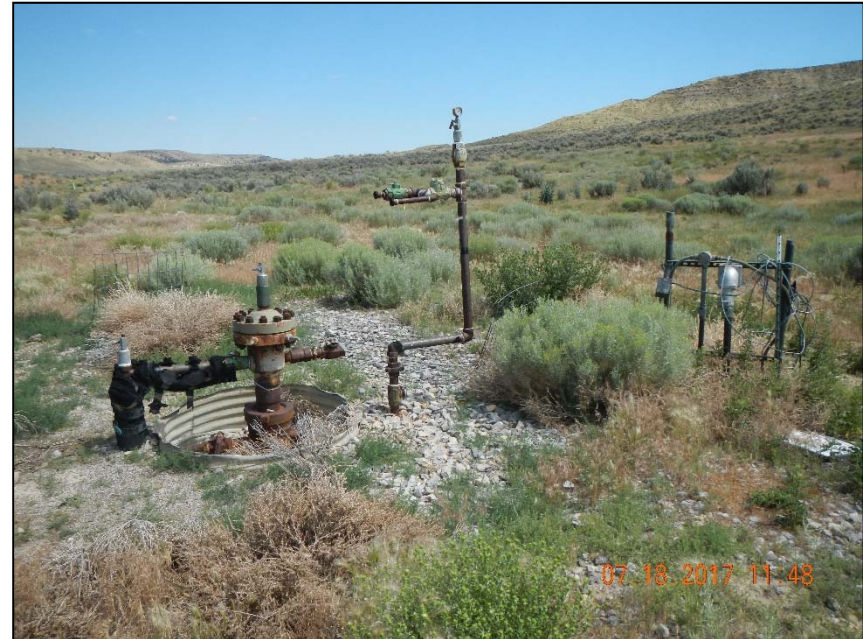
Photo 3. Unused 2" steel riser at wellhead.
