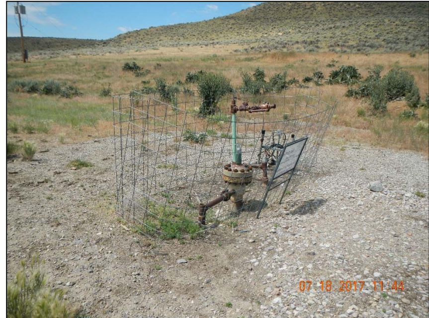
Photo 3. Unused 2" steel riser at wellhead.
