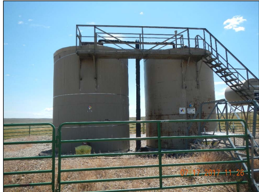
Photo 3. Incomplete or missing tank labels.
