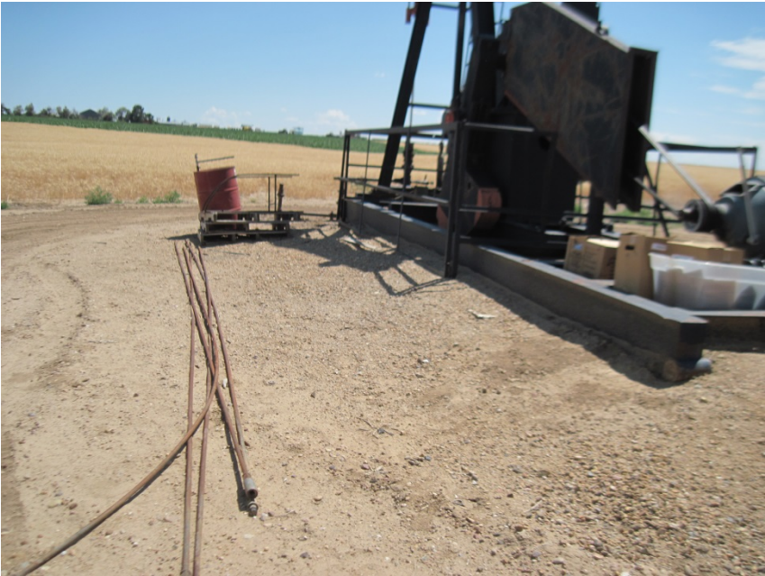
UNUSED EQUIPMENT SUCKER RODS AND PALLETS
