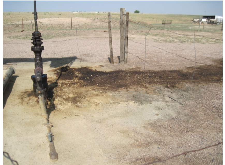
Stained soil around wellhead
